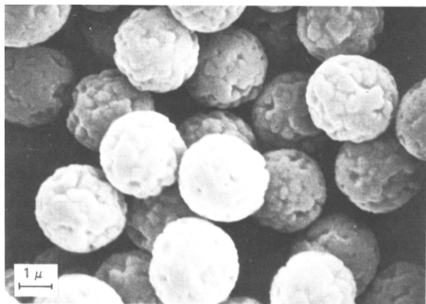
Fig. 1. Scanning electron micrograph of the crosslinked polystyrene particles used in this study.
